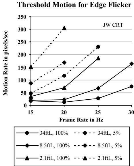
**Fig. 2** The results for observer JW for motions viewed on a CRT. Three brightness levels and two contrast conditions are shown. Each curve is labeled by the brightness in ftL and the nominal Michaelson contrast.
