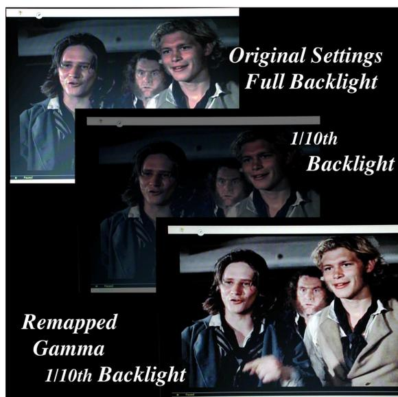
Fig. 6 A video scene rendered on a prototype display with 3 different setting combinations.
