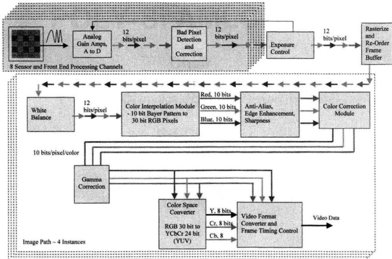
Figure 2 – Camera Electronics Architecture
